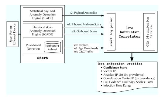
**Figure 6:** BotHunter system architecture.
