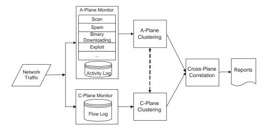
Figure 20: Architecture overview of our BotMiner detection framework.
